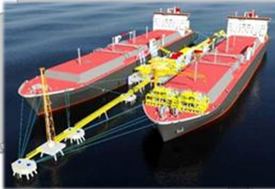
Offshore LNG Terminal using Double-Berth Floating Storage & Regasification Unit (FSRU) Technology [Illustration photo]
